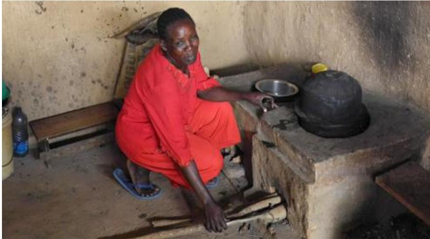
This picture is sourced from myclimate ETH Zurich project document. This efficient stove has a cleaner, more efficient combustion and better heat insulation, which reduces smoke emissions and firewood consumption significantly.
